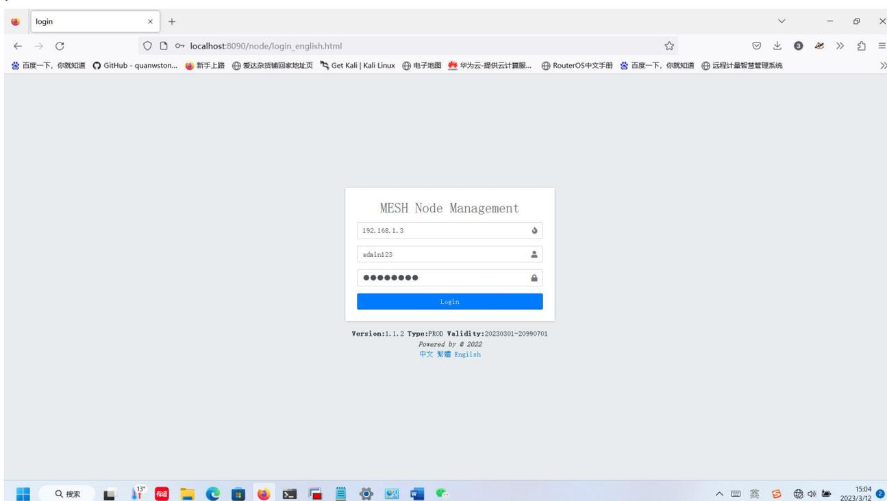
Input the IP address of each node, user name(admin123) and password(admin123), you can access the configuration.
