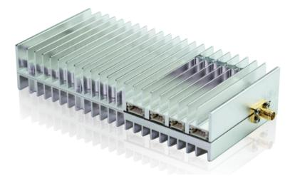
FDM-615PTM is a point to multi-point network board for long range video and data downlink to ground. It supports multi transmitters in air sending HD video and TTL data to one receiver on ground. It is special designed for fixed wing drone/helicopter/Vehicles video downlink for 100km-150km during fast moving.
